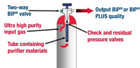
Our patented BIP<sup>®</sup> technology features not only an automatic shut-off valve but also a non-return valve making it impossible for any external contamination to enter the cylinder. Perfect gas quality is therefore guaranteed every time giving you peace of mind and allowing you to concentrate on your business.
