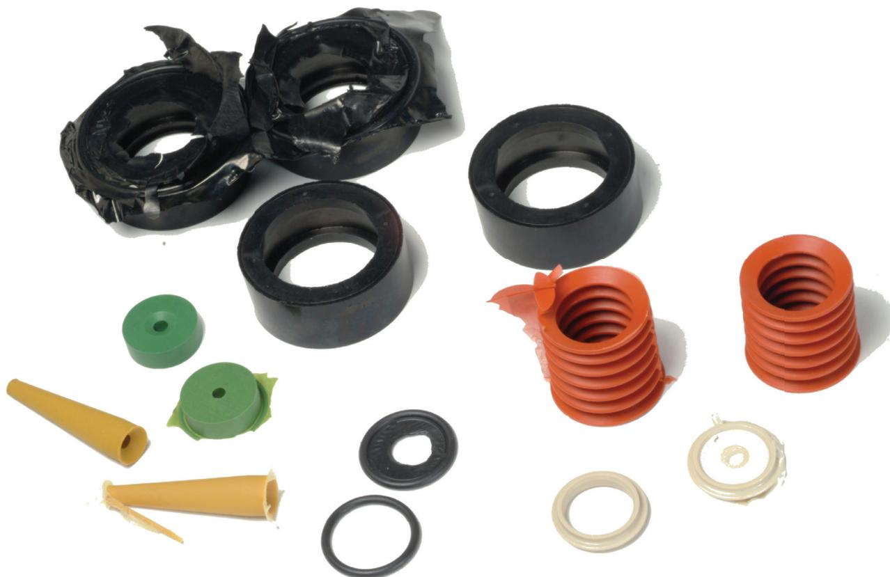
As industries continue to push the envelope towards more sophisticated and intricate molded parts, and manufacturers strive to safely comply with increasingly rigorous quality standards, cryogenic deflashing is a viable solution that balances both needs while maintaining efficiency and productivity in the manufacturing process.
