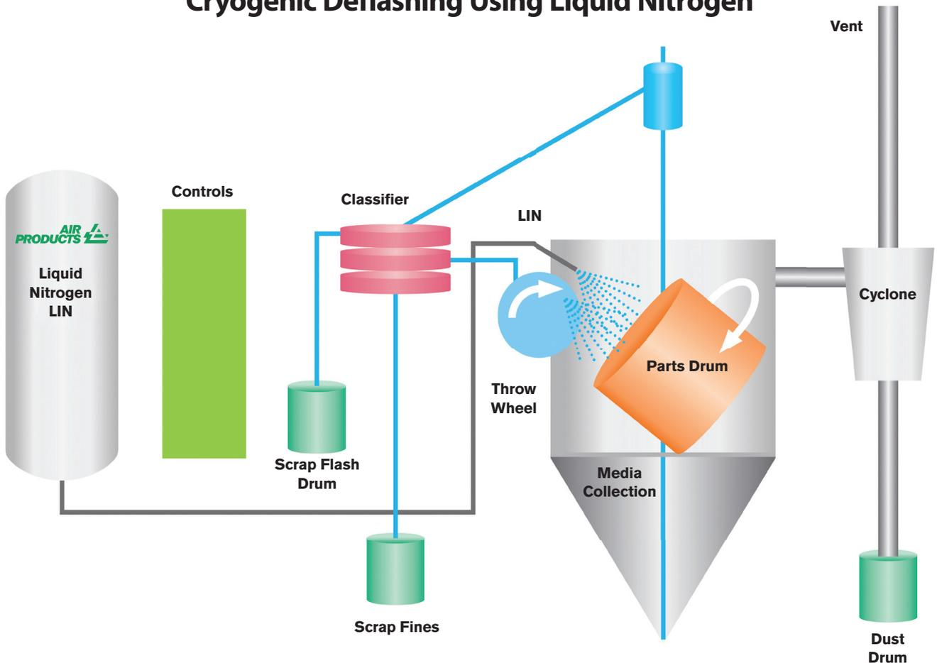
This schematic depicts a cryogenic deflashing process using liquid nitrogen. Using the very low temperature of cryogens like liquid nitrogen, cryogenic deflashing temporarily embrittles residual material for removal when subjected to stress applied through tumbling and media blasting.
